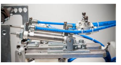
In the leak tests using the pressure decay method, even the smallest leaks are detected by monitoring the compressed air in the product at the level of 0.1 Pa. Adlema BT4000 series devices automatically decide if the tested products are OK/NOK. In this way, subjective test results originating from the operator are not encountered. Thanks to its reportability feature, you can examine the leak testing performance of your products and keep records.
